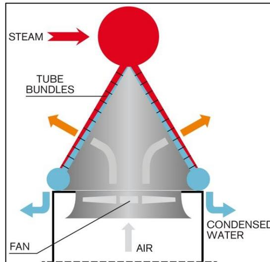
Figure 9: Dry Cooling Tower (Bushart, 2014)
