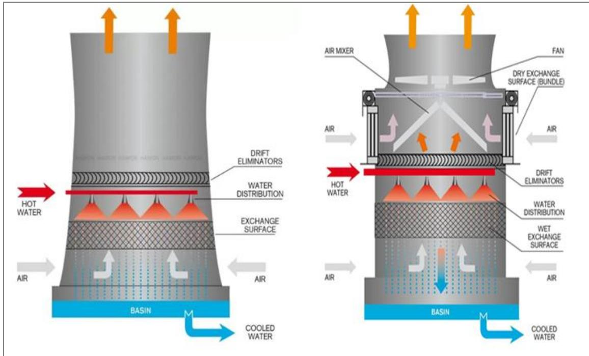
Figure 8 (a): Natural draft cooling tower (b): Induced draft cooling tower
