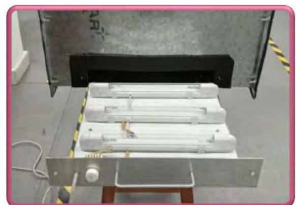
Figure 16 :UV-C retrofit module
