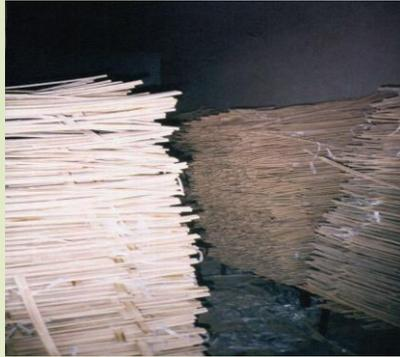
1. Bamboos are split into thick section (or sheets)
