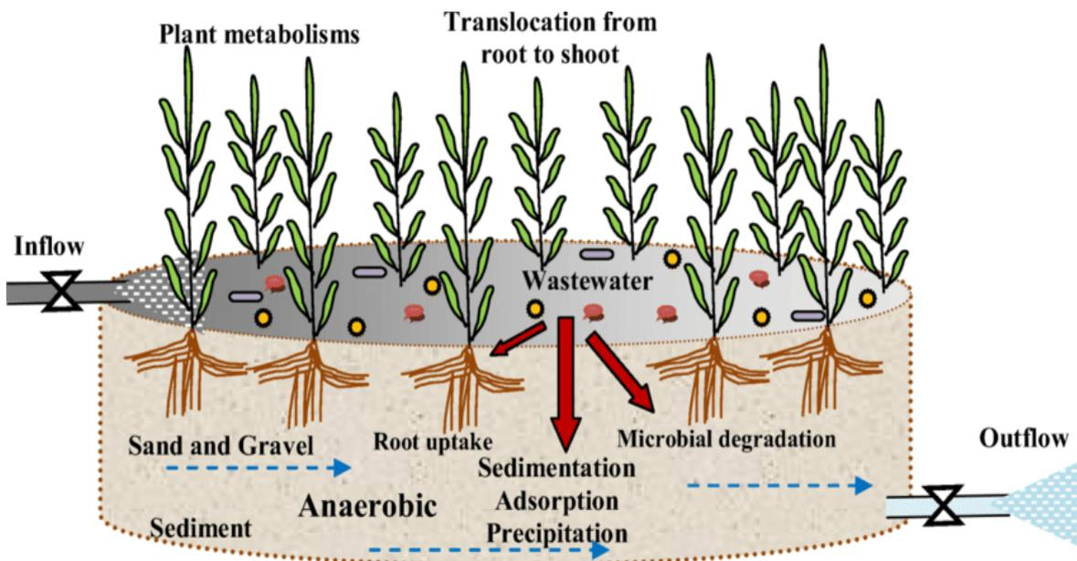
Figure 4.2.2: Pollution removal mechanism for constructed wetlands
