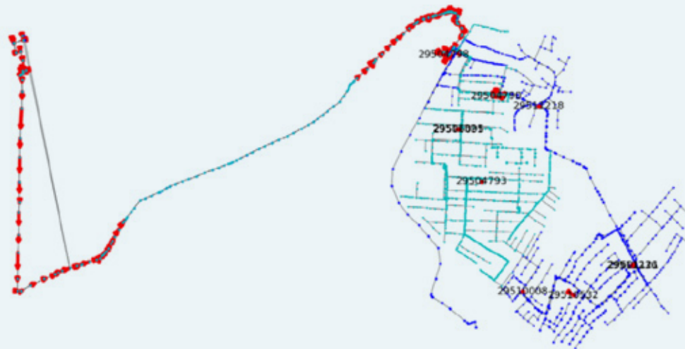
Figure 6.33: Line loading due to high EV penetration. Overloaded line segments are shown in red 177
