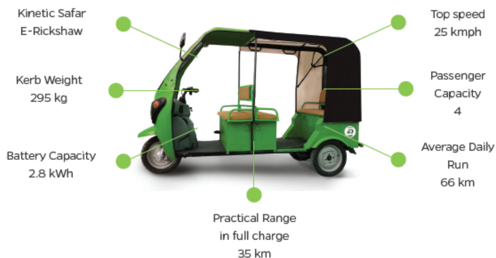
Figure 6.10: Features of e-rickshaw in the project 129
