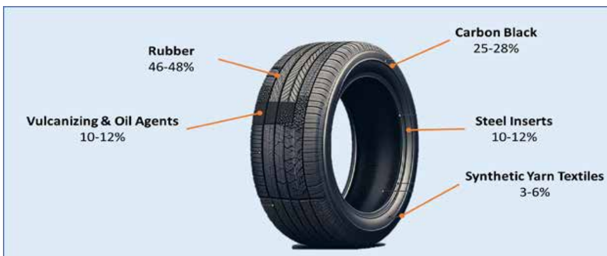
Figure 1: Components of a Tyre
